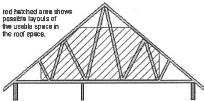
Roof trusses are frequently used in the construction of slanted roofs to stabilize shifting weight that they are subject to in the course of their lifetime. The roof you are sitting under right now may be subject to snow that piles up on top of it, or wind that hits it from one direction or another. The truss makes sure that the changing forces that the roof may encounter (known by architects as **live load**) won't cause it to shift or collapse.
